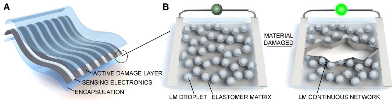
Figure 1. A) Sensing architecture consisting of an active damage layer of LM composite with LM sensing electronics encapsulated in soft elastomer. B) Schematic showing the structure of the active damage layer with LM droplets are dispersed in an elastomer matrix. Prior to damage the droplets are isolated and the material is electrically insulating. C) When damage is induced the LM droplets rupture, connect together forming a percolated, electrically conductive network.
