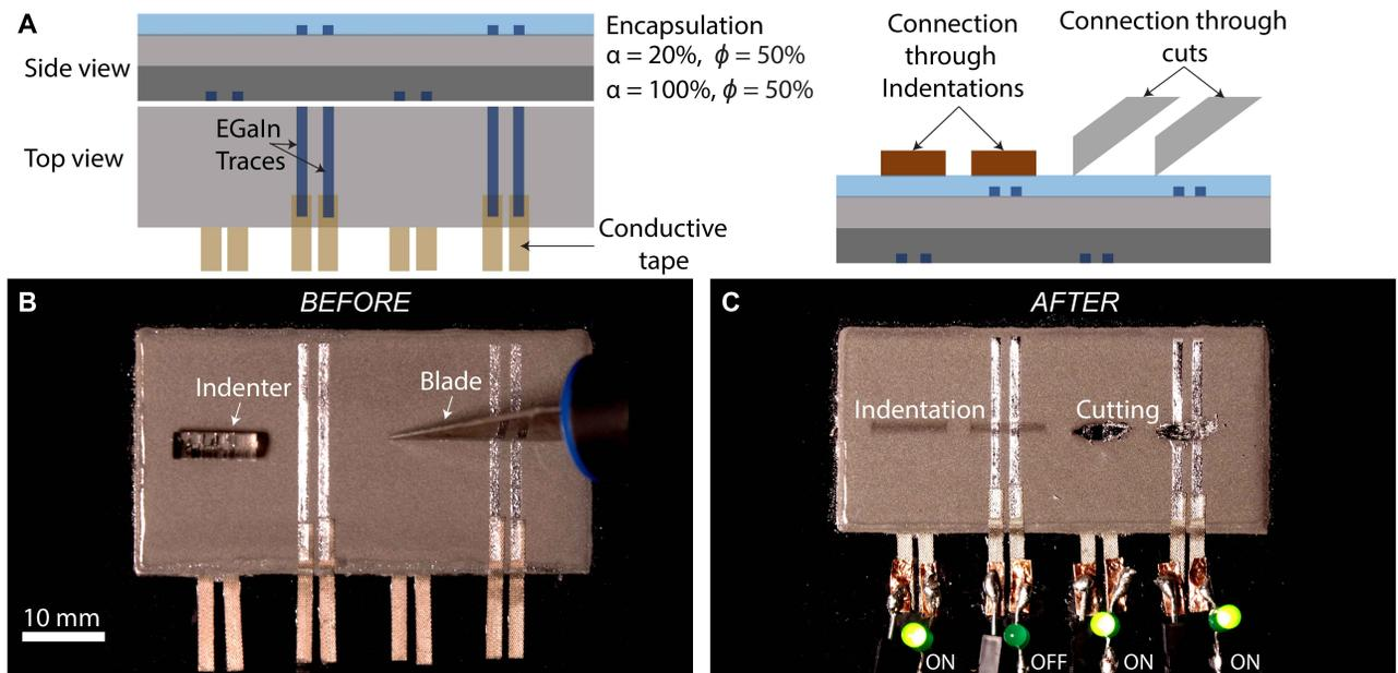
Figure 4. A) Damage selectivity architecture. B) Material before damage and C) Material after indentation and cutting damage with selectivity where compression is sensed when only one LED turns on, and cutting when both turn on.
