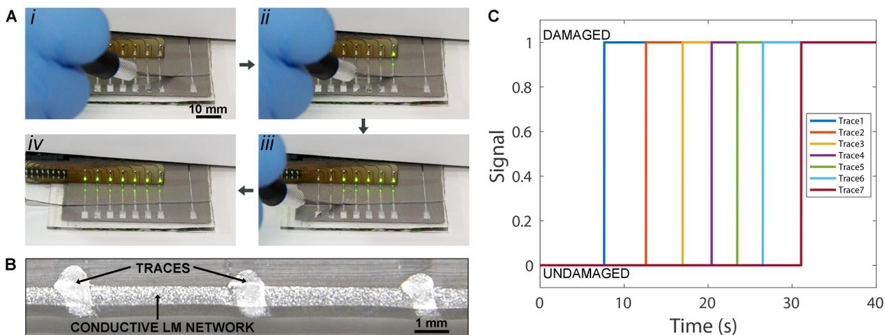
Figure 2. A) Time sequence showing the cutting of a film and damage indication by LEDs. B) Cross-sectional micrograph showing the conductive LM networks upon damage which are sensed by the LM traces. C) The damage detection signal as a function of time as the knife moves across the sensing array.
