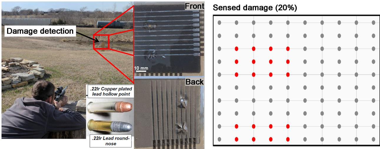
Figure 3. Multiple ballistic damage points identified, quantified (plot), and communicated in real-time. The front and back images show the damage inflicted in the soft matter damage detection system with ballistic impact.
