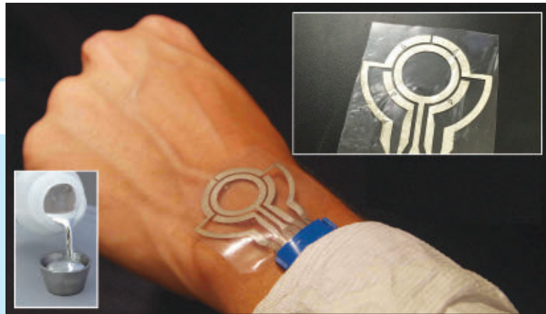
FIGURE 2 Tactile sensor with laser-patterned traces of eutectic gallium-indium (EGaln) liquid metal (LM) embedded in silicone elastomer.
