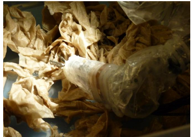
Figure 6. Benchtop Testing: Dampened Paper Towels Used to Simulate a Semi-Aqueous Surgical Environment.
