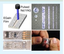
to wearable computing and biosensing are demonstrated with functional implementations in which soft-matter PCBs are populated with surface-mounted microelectronics.
