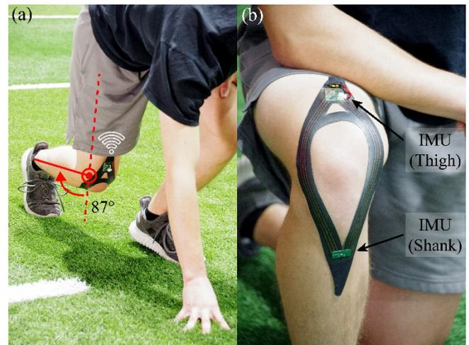
**FIGURE 1: (a)** THE FULLY UNTETHERED AND STRETCHABLE, WEARABLE ELECTRONIC BANDAGE IS SHOWN ATTACHED TO THE KNEE FOR MEASURING KNEE MOTION. **(b)** THE WEARABLE DEVICE CONTAINS AN INERTIAL MEASUREMENT UNIT (IMU) LOCATED ON THE THIGH AND SHANK. DURING OPERATION, MOTION DATA IS COLLECTED FROM EACH SENSOR, THE DATA IS WIRELESSLY TRANSMITTED TO A NEARBY COMPUTER, AND JOINT ANGLE IS ESTIMATED.
