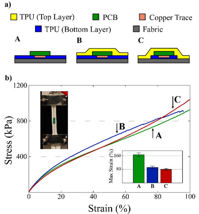
**FIGURE 3: (a)** CROSS-SECTIONAL ILLUSTRATIONS OF THE DIFFERENT CONFIGURATIONS (A, B, C) OF THE ELECTRONIC BANDAGE. **(b)** MEAN STRESS VERSUS STRAIN UNDER UNIAXIAL DEFORMATION OF THE 3 DIFFERENT CONFIGURATIONS (A, B, C) SHOWN IN 3(a) **(LEFT INSET)** PHOTOGRAPH OF DOG-BONE SAMPLE DURING UNIAXIAL DEFORMATION TESTING **(RIGHT INSET)** ELECTRICAL FAILURE STRAIN FOR THE DIFFERENT CONFIGURATIONS SHOWN IN 3(a).
