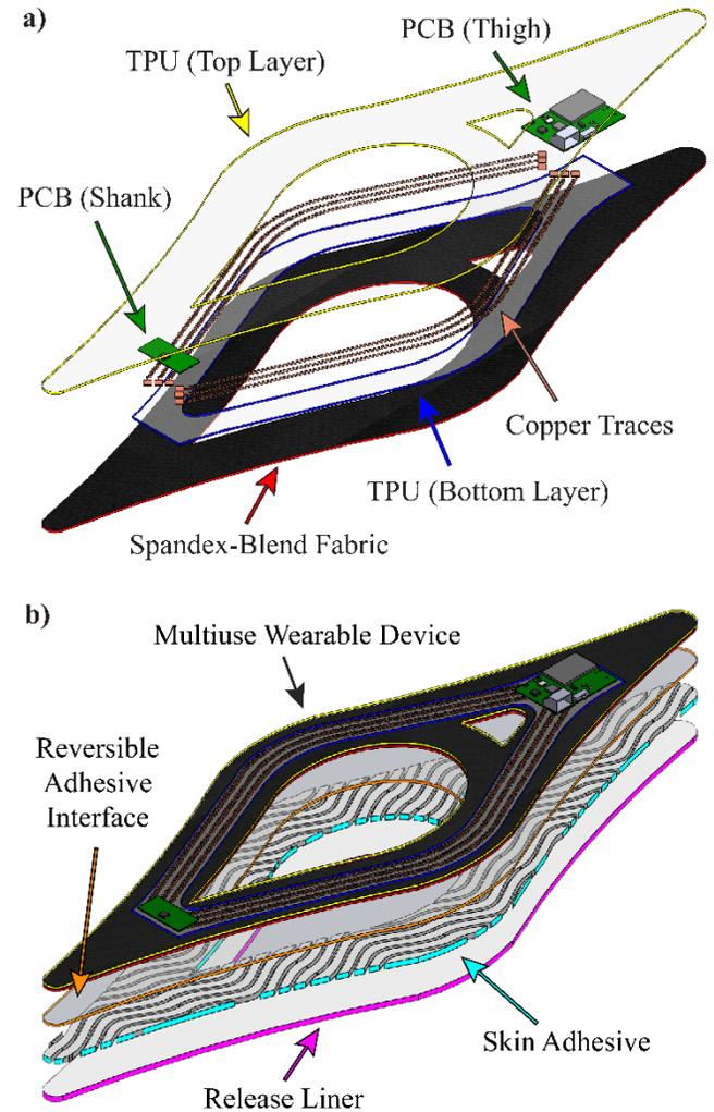
**FIGURE 2:** (a) EXPLODED VIEW OF THE MULTIUSE WEARABLE DEVICE FOR MEASURING JOINT-LEVEL HUMAN MOTION OF THE KNEE. (b) EXPLODED VIEW OF THE REPLACEABLE SKIN ADHESIVE THAT CAN REVERSIBLY ATTACH TO THE WEARABLE DEVICE UTILIZING A REVERSIBLE ADHESIVE INTERFACE.
